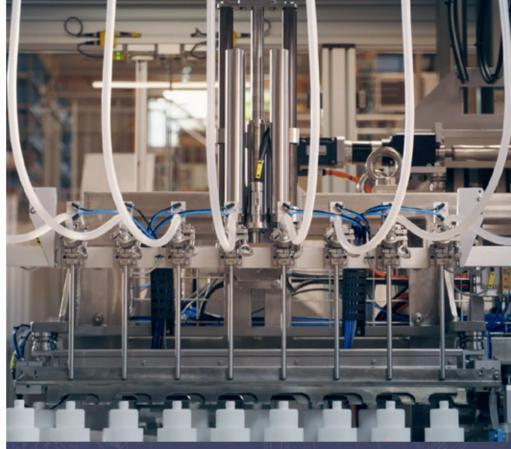
The LinMot SM01 and SM02 guides are manufactured from 316L stainless steel, which is recognised as the standard in the food, pharmaceutical and chemical industries. This is particularly important in filling systems where strict hygiene standards are essential.
