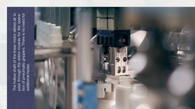
"The Z-axis must also be designed by the machine builder. This is a very complex challenge for the screwing process of our products, as they are offered in a wide variety of formats, all of which have to run on this one machine," says Mr Vaas, addressing a common problem for many machine builders. For this reason, LinMot offers the PR02 linear rotary motor for linear rotary motion, which, unlike competing products, is an all-in-one solution that meets the var-
