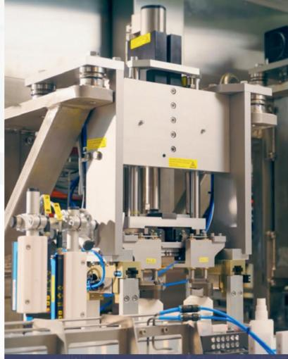
LinMot actuators provide high repeatability, ensuring that each part is placed in exactly the right place, which is essential when placing the caps.
