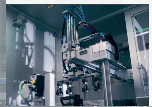
strength classes, sizes, stroke lengths and a comprehensive range of accessories, as well as stainless steel versions and stroke lengths of up to 2 metres, LinMot linear guides and modules offer exceptional performance in any production environment and machine integration.
